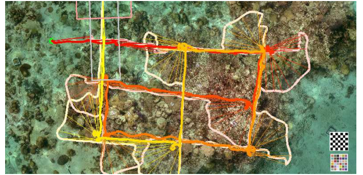
Fig. 3. Robot path over the poster, as estimated from the homographies. The bright line shows the camera movement, the saturated the robot center.
